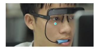
**Description**: Head tracking device for adaptive control phone, tablet, or computer; Can be used on it's own or with
